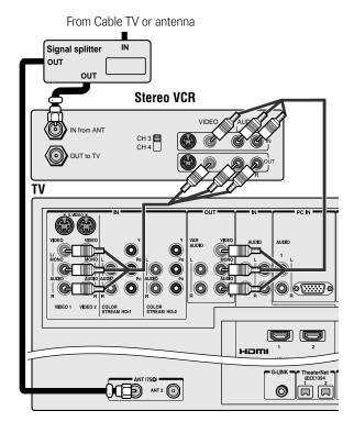
**Note:** The VIDEO/AUDIO OUT terminals output signals from the ANT 1, ANT 2, VIDEO 1, VIDEO 2, and VIDEO 3 terminals when the appropriate input mode is selected.
